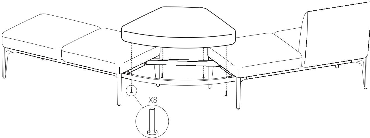
**EN** - 1) Fasten the central leg to the curved frame by using the supplied screws.
