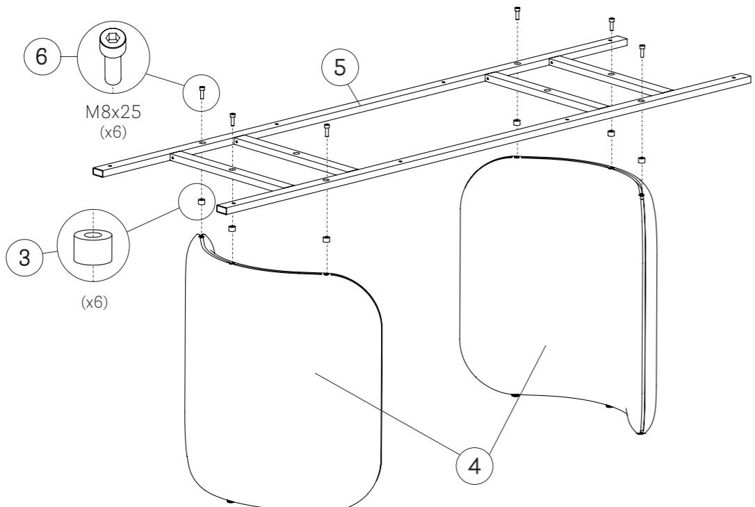
**EN** - Insert the spacers (3) between the bases (4) and the metal frame (5) fixing them with the supplied screws (6).
