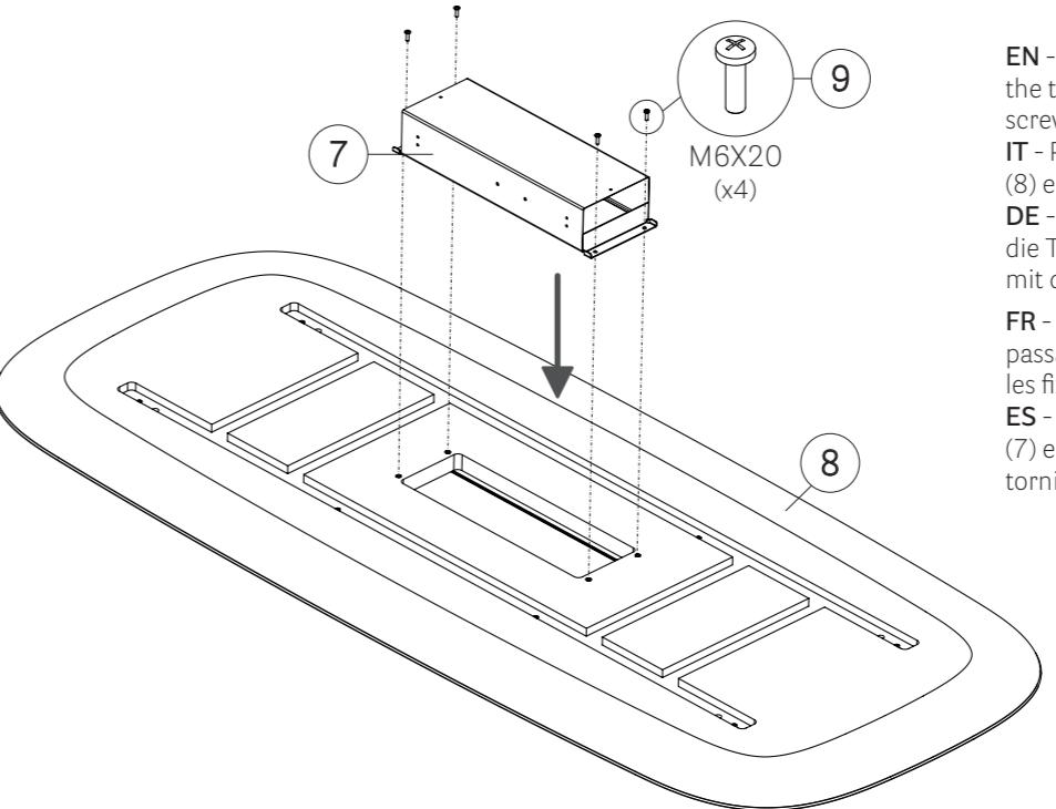
**EN** - Place the cable management (7) on the table top (8) and fix them by means of screws (9).
