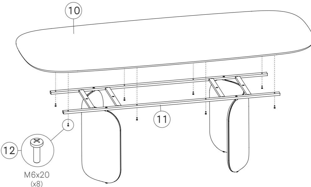
**EN** - Fix the top (10) on the metal frame (11) using the supplied screws (12). If necessary, adjust the feet to stabilise the table.
