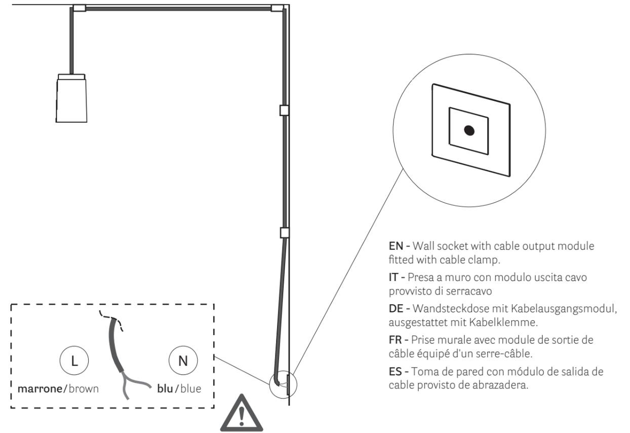
**EN** - Wall socket with cable output module fitted with cable clamp.
