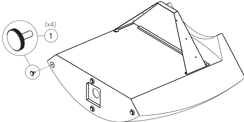
**EN** - Install and adjust the gliders included in the Kit (1) under the IGLOO CORNER bar counter.
