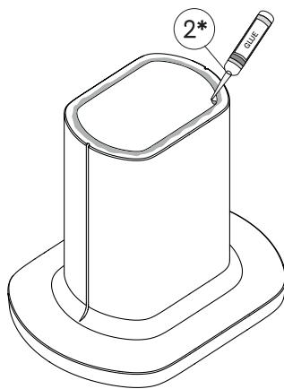
**EN** - Equip yourself with protective gloves and adhesive sealant (2\*). Spread a thin strip of sealant on the base near the innermost perimeter.
