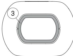
**EN** - Press down vertically on the foot until it is completely adhered, taking care not to slide it on the surface. **⚠** Wait 24 hours before turning over and using the table.
