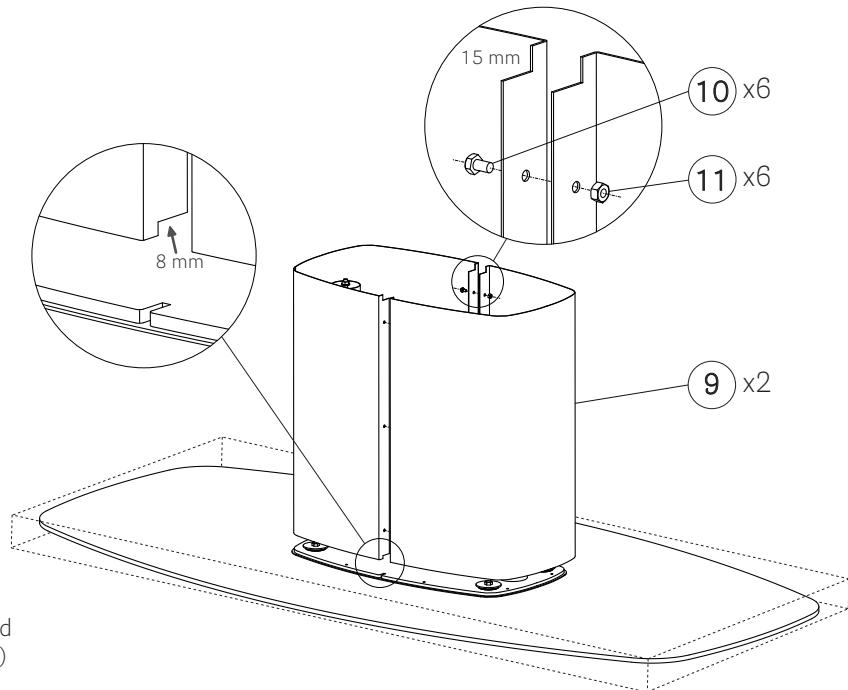
**EN** - Put the base (12) on the rod bars and covering and fix it through the flanged nuts (13). Tighten screws (10) and nuts (11) using the opening on the base (12).
