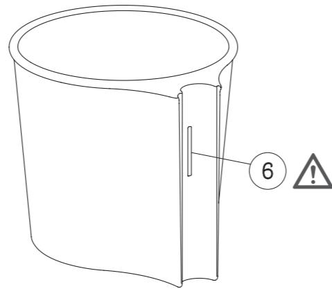
**EN** - Place the concave surface of the pot holder, starting at its bottom, on the tube. Hang the pot holder on the hook, inserting the hook into the hole. Complete assembly by pressing the pot holder downwards into a vertical position. Carry out the same operations for the remaining potholders.
