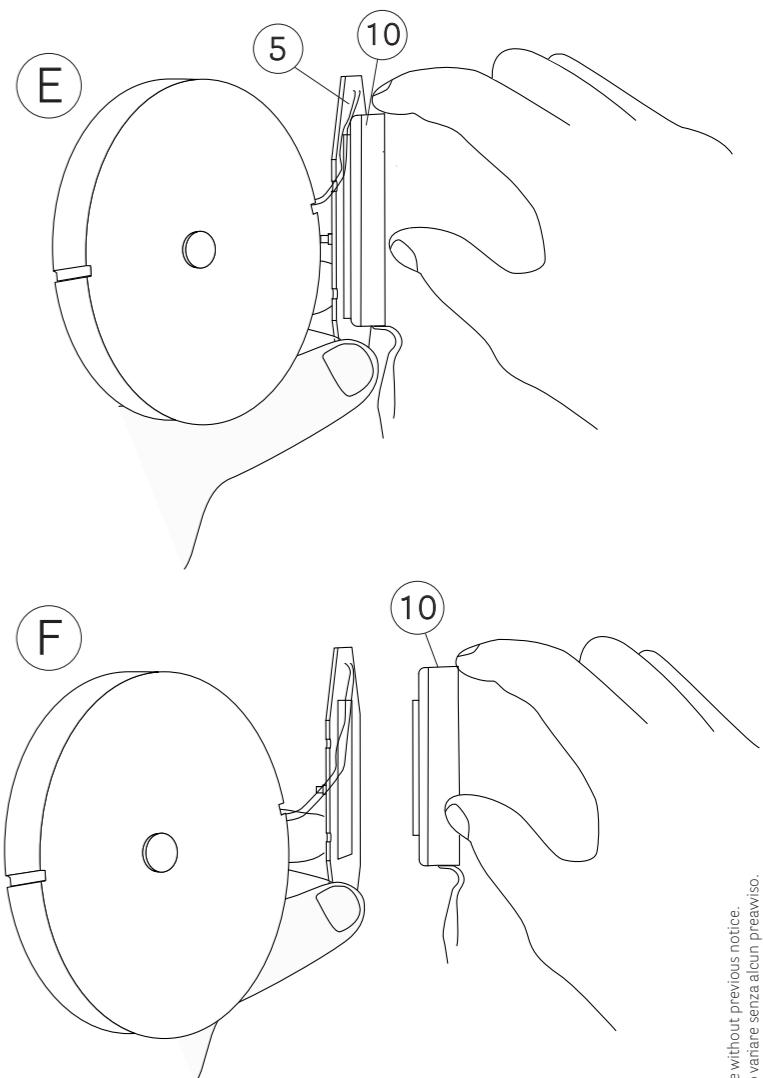
**EN - (F)** Install the provided battery (10) and reassemble the lamp carrying out the following steps:
