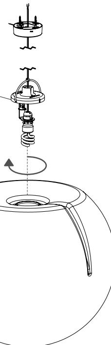
EN - (A) Unscrew the diffuser (2) from the light kit (1).
