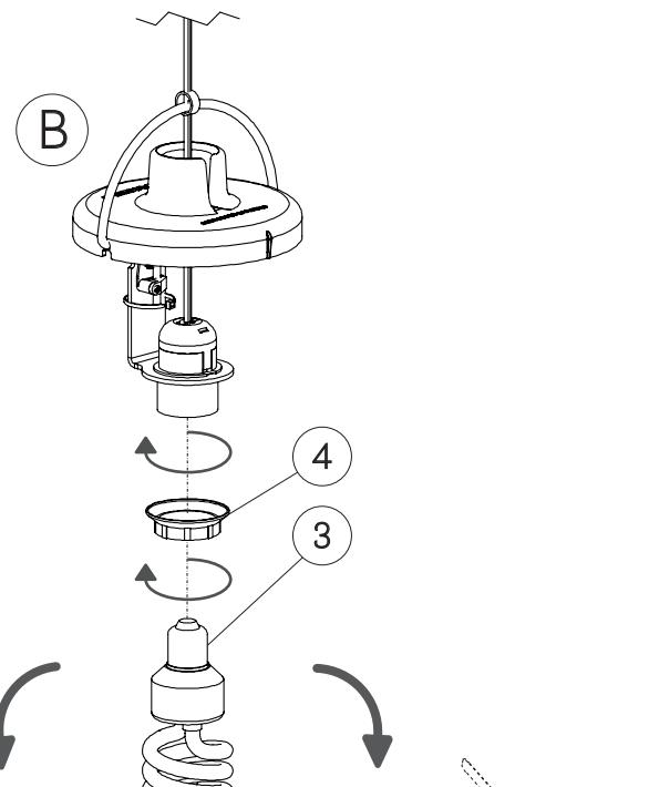
EN - (B) Unscrew both bulb (3) and locking ring (4). Pull the bulb holder (5) out of the housing (6) and insert first the washer (7) and then the supplied support plate (8).
