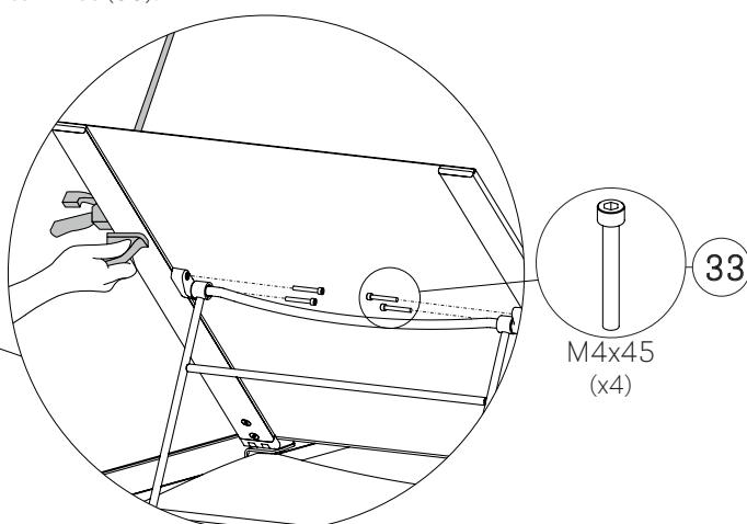
**EN** - Lower the backrest and turn the sun lounger upside down. Fasten the bed base to the frame with the screws (34).
