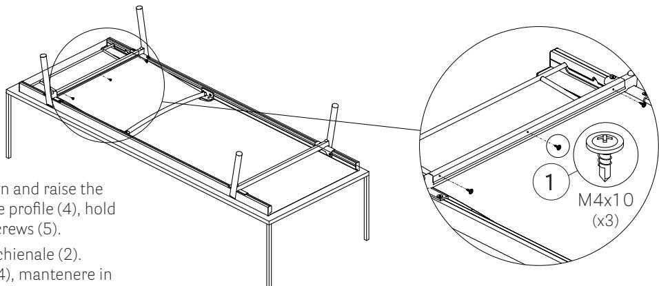
**EN** - Turn the sun lounger upside down and raise the backrest (2). Place the clamp (3) on the profile (4), hold under slight tension and remove the screws (5).
