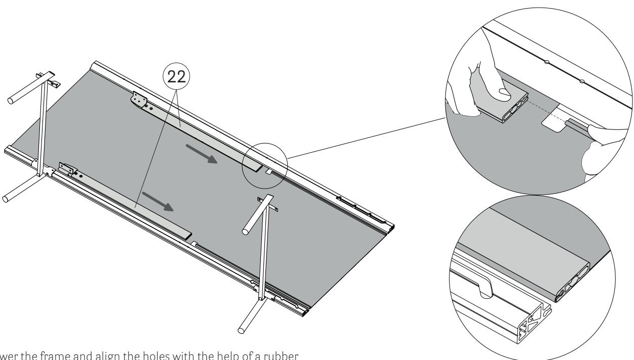
**EN** - Lower the frame and align the holes with the help of a rubber mallet and position the clamp.
