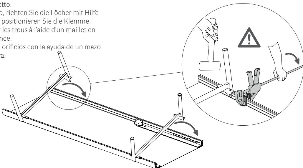
**EN** - With slight tension on the clamp, insert screws (23) and (24).
