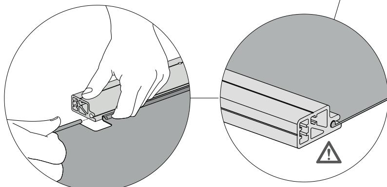
**EN** - Slide the extruded parts of the reclining backrest (22) along the edge of the net as they are flush.
