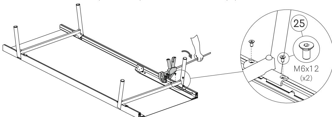
**EN** - Position the clamp by tensioning the frame and position the backrest net (26) by aligning the holes.
