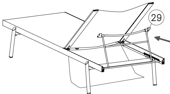
**EN** - Place the clamp between the backrest profiles (30) under slight tension and slide the frame down until it is aligned with the holes.
