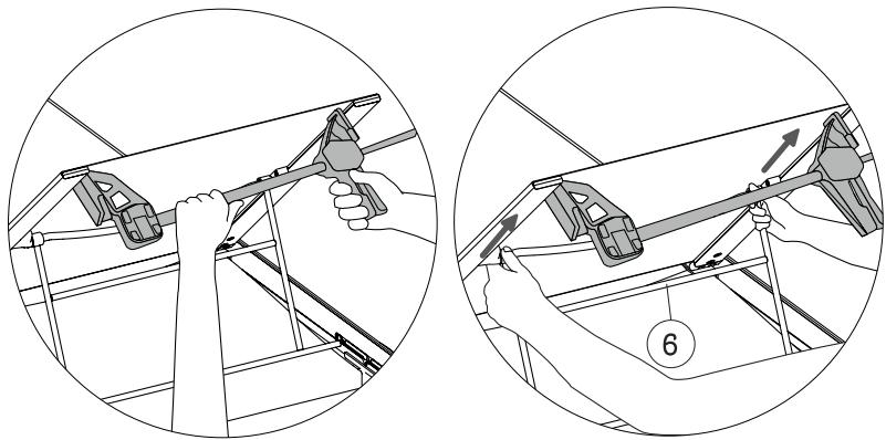
**EN** - Turn the sun lounger upside down and position the clamp by tensioning the frame (7), remove the screws (8) and remove the backrest net (9).
