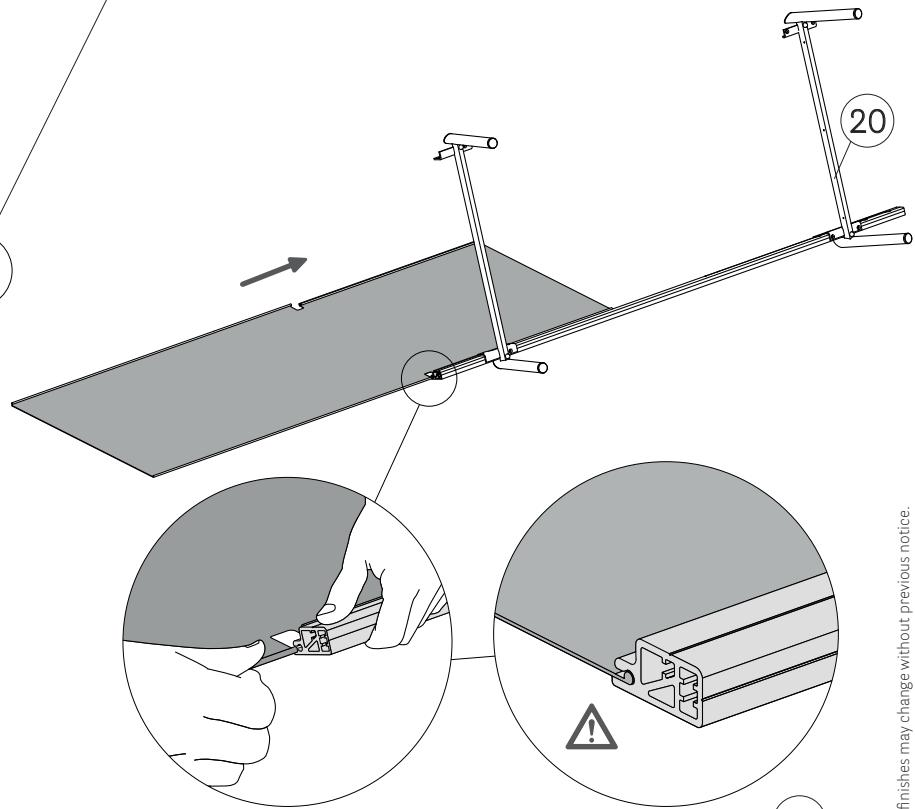
**EN** - Insert the net edge into the frame profile (20) and slide until it is flush.
