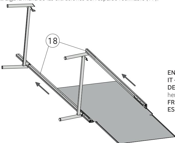
**EN** - Pull the net out of the frame extrusions (18).
