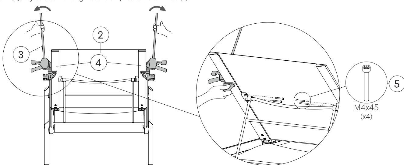
**EN** - Place the clamp between the two aluminium profiles of the backrest under slight tension and remove the frame of the reclining backrest (6).
