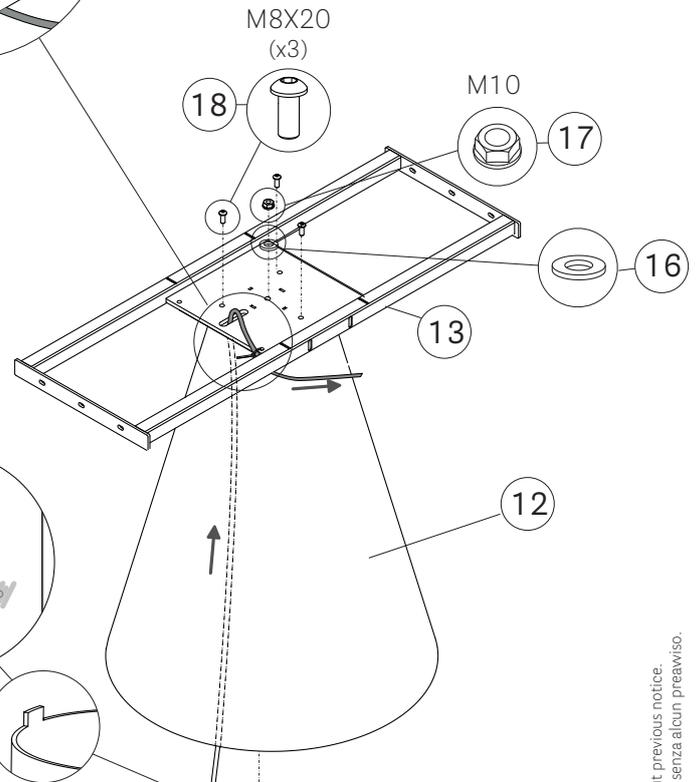
**EN** - Insert the teeth into the corresponding slots of the cross
