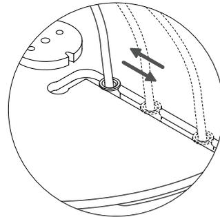
**EN** - Position the cross (5) on the column (6) and mark the position of the hole at the slot with a felt-tip pen. Make a hole in the column to run the cable through.
