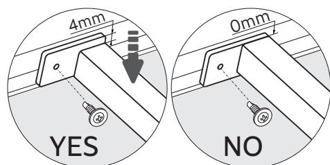
**EN** - Self-tapping screw - Use automatic screwdriver
