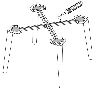
**EN** - Place the top on a smooth and anti-scratch surface, turn the tablebase upside down centering the sleeves to the holes of the cross. Screw the crews to the top by hand. Let the adhesive sealant dry for 48 hours without moving or touching the table. Remove the centring screws after gluing.
