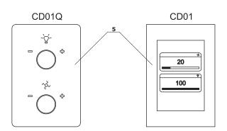
Note: Acoustic booth with faster production time - control panel with manual (knobs) adjustment of lighting and ventilation
