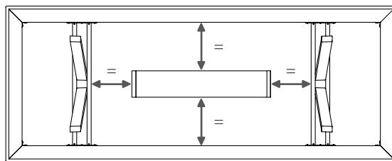
**EN** - Fit the crosspieces (5) to the cable management (4) and fix them to the structure (1) by means of screws (6).
