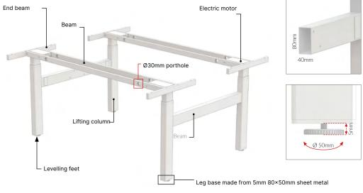
Beam linking lifting columns made from 1.5mm 80×40mm tube, screws to the columns.
