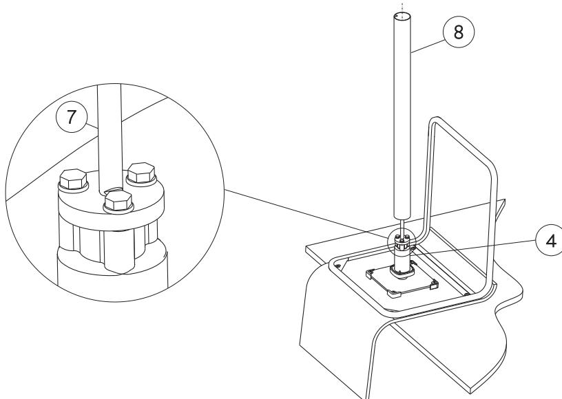
**EN** - Remove the protecting pvc film from the cover base (9) and together with the base (10) put it into the tube (8), keeping a parallel alignment between one side of the base and the back of the shell. Insert the washer (11), the locking nut (12) and tighten the lock nut (13).
