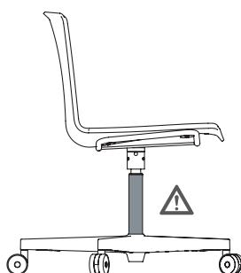
**EN - !** Only trained personnel may replace or repair seat height adjustment components with gas lift columns.
